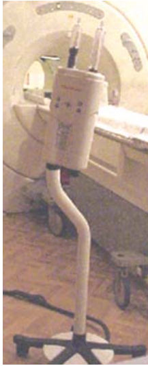
Fig. 3.8: MR compatible contrast media injector (Med Rad)
