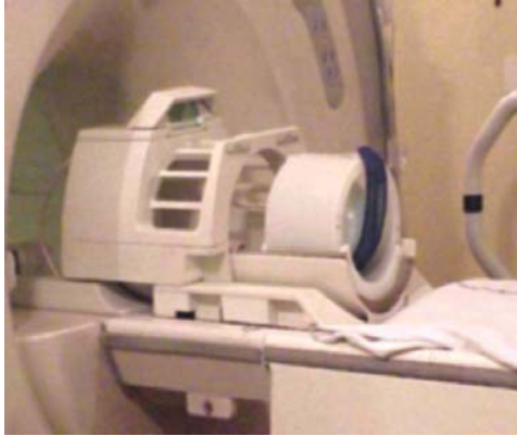
Fig. 3.10A: Phantom placed in the head coil
